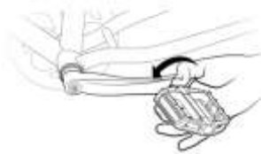
Thread the left pedal onto the left crank gently by hand, turning counterclockwise.
