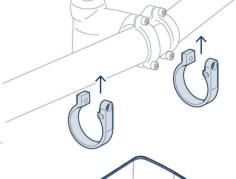
2 > Install the display on the support, tightening the M4 fixing screws.
