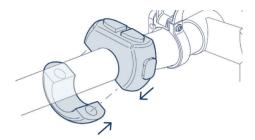
2 > Tighten the fixing screws.
