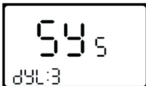
Delay time of battery power interface
